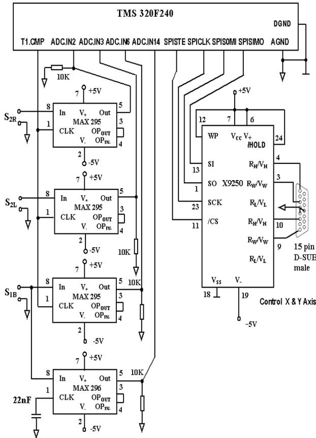
**Figure 4.** Schematics for anti-aliasing filter, DSP and digitally-controlled potentiometers
