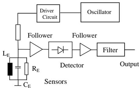
**Figure 2.** Block scheme of the sensor and circuitry used to drive it
